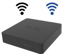
PIXIE Gateway connects to in-home WiFi or modem directly via RJ45 port and acts as a bridge between the internet, PIXIE Cloud and the PIXIE device's Bluetooth mesh in home.
