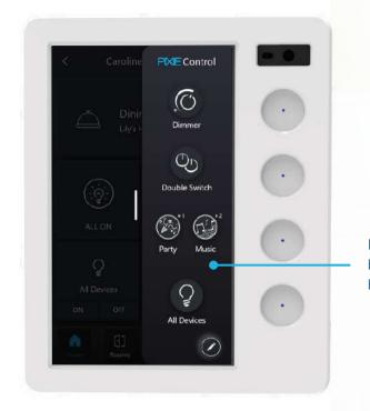
Pull out menu acts as a reminder of button functions and fast multifunction button re-configuration tool.
