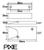
For garage door and gate status functionality, including push notifications to mobile devices, it's necessary to install the roller door contact sensor (CSR41BTP) and have it connected to the PIXIE garage door and gate controller.
